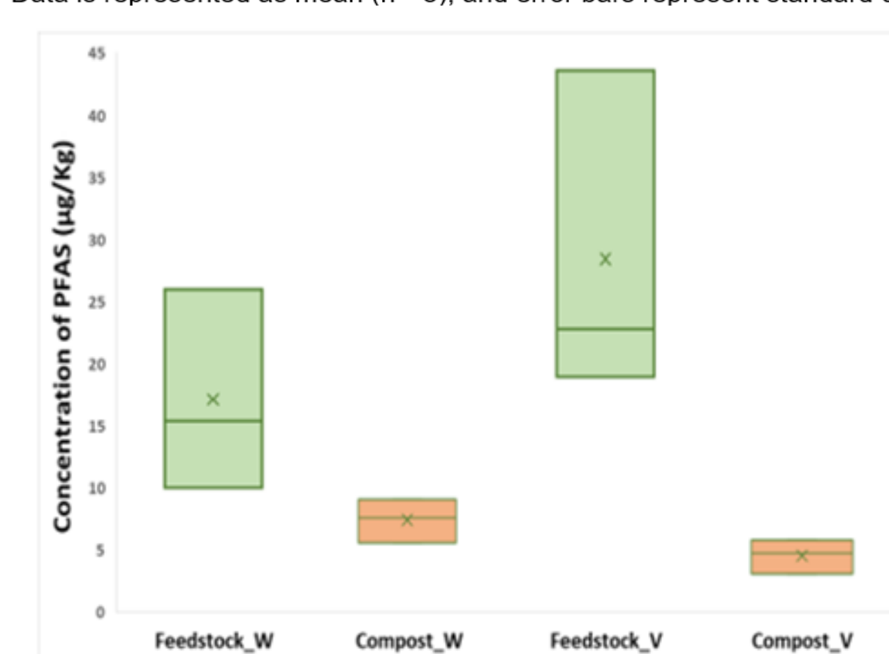
Figure 4: The sum of PFAS concentration of solid samples ( \mu\text{g/kg} ) from: a. Windrow (Feedstock_W, and Compost_W) and In-vessel composting systems (Feedstock_V, and Compost_V). Data is represented as mean ( n=3 ).
